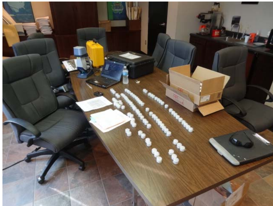
Photo 16: Scanning samples with an X-ray fluorescence system (XRF).
