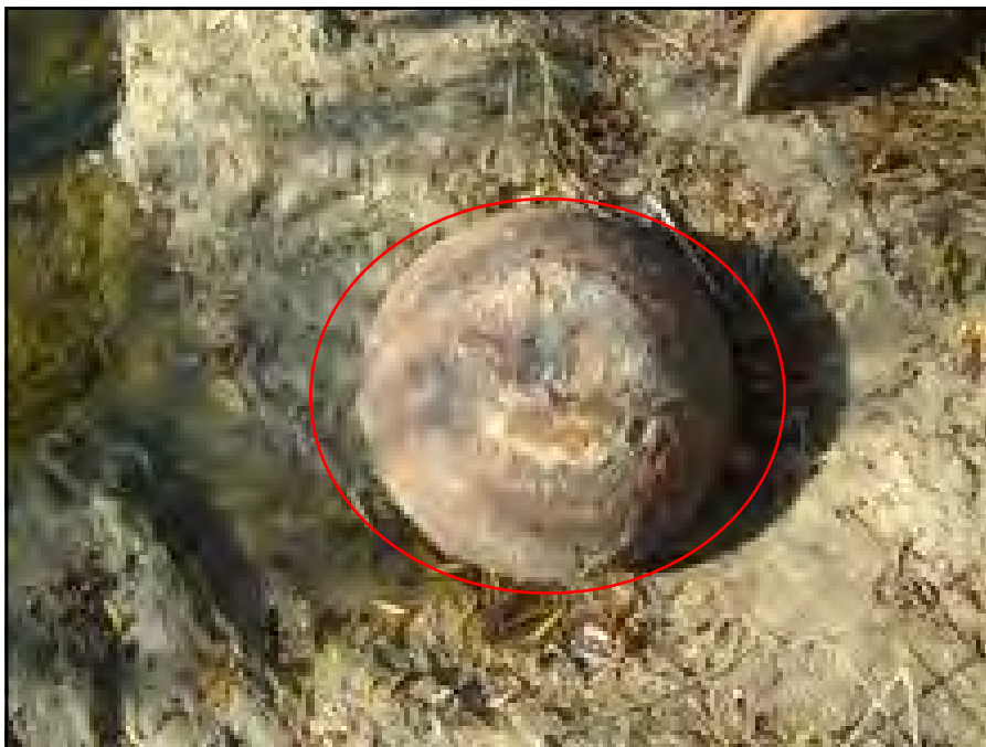
Photo 5: Sample 112-041-SL-05. Identified as slag based on test results.
