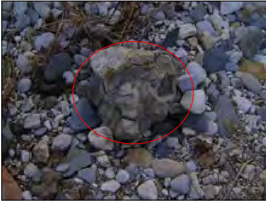
Photo 9: Sample 112-041-SL-10. Not identified as slag based on test results.
