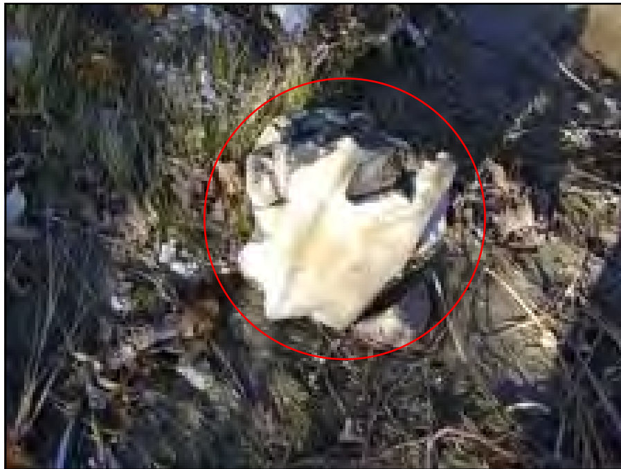
Photo 4: Sample 112-041-SL-04. Not identified as slag based on test results.
