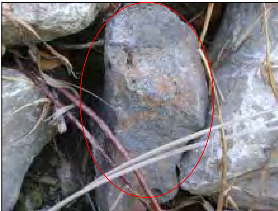
Photo 1: Sample 112-041-SL-01. Identified as probable slag based on test results.
