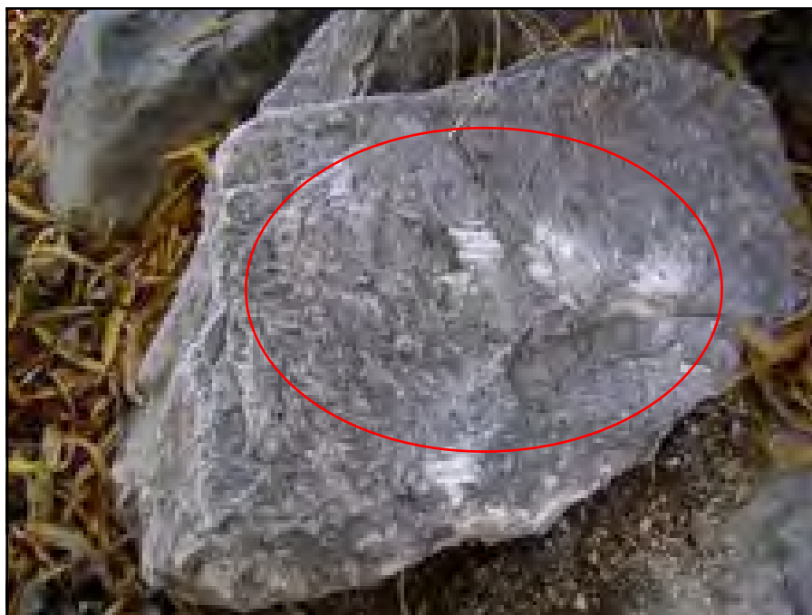
Photo 2: Sample 112-041-SL-02. Not identified as slag based on test results.
