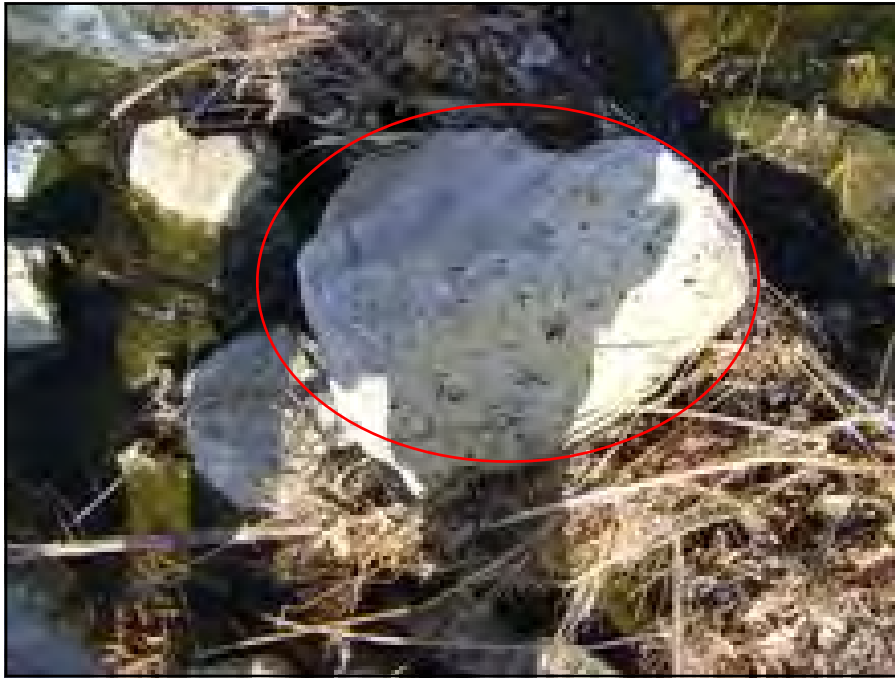
Photo 3: Sample 112-041-SL-03. Not identified as slag based on test results.
