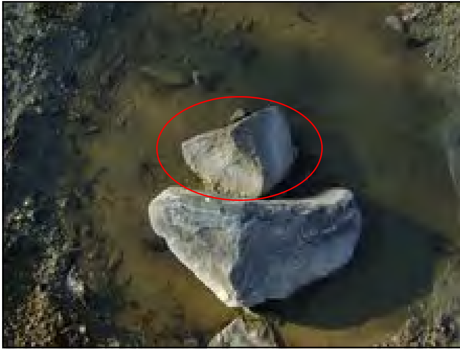
Photo 7: Sample 112-041-SL-07. Identified as slag based on test results.
