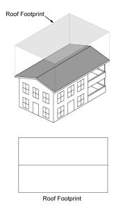
the water coming off the valley of your roof to fill your barrel. It is important to understand that you will not likely be able to harvest all of the rain that falls onto your roof, nor is it necessary in home applications. Above
