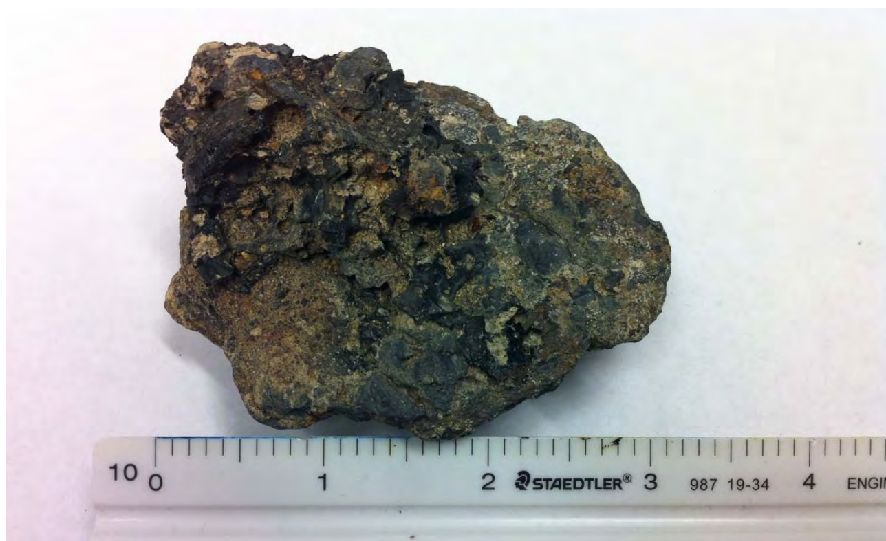
9.) Photo of potential slag observed near the Dallas North Tollway Bridge.
