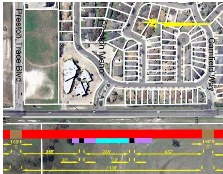
Figure 8 – Scenario 1 with Unacceptable Driveway Spacing
