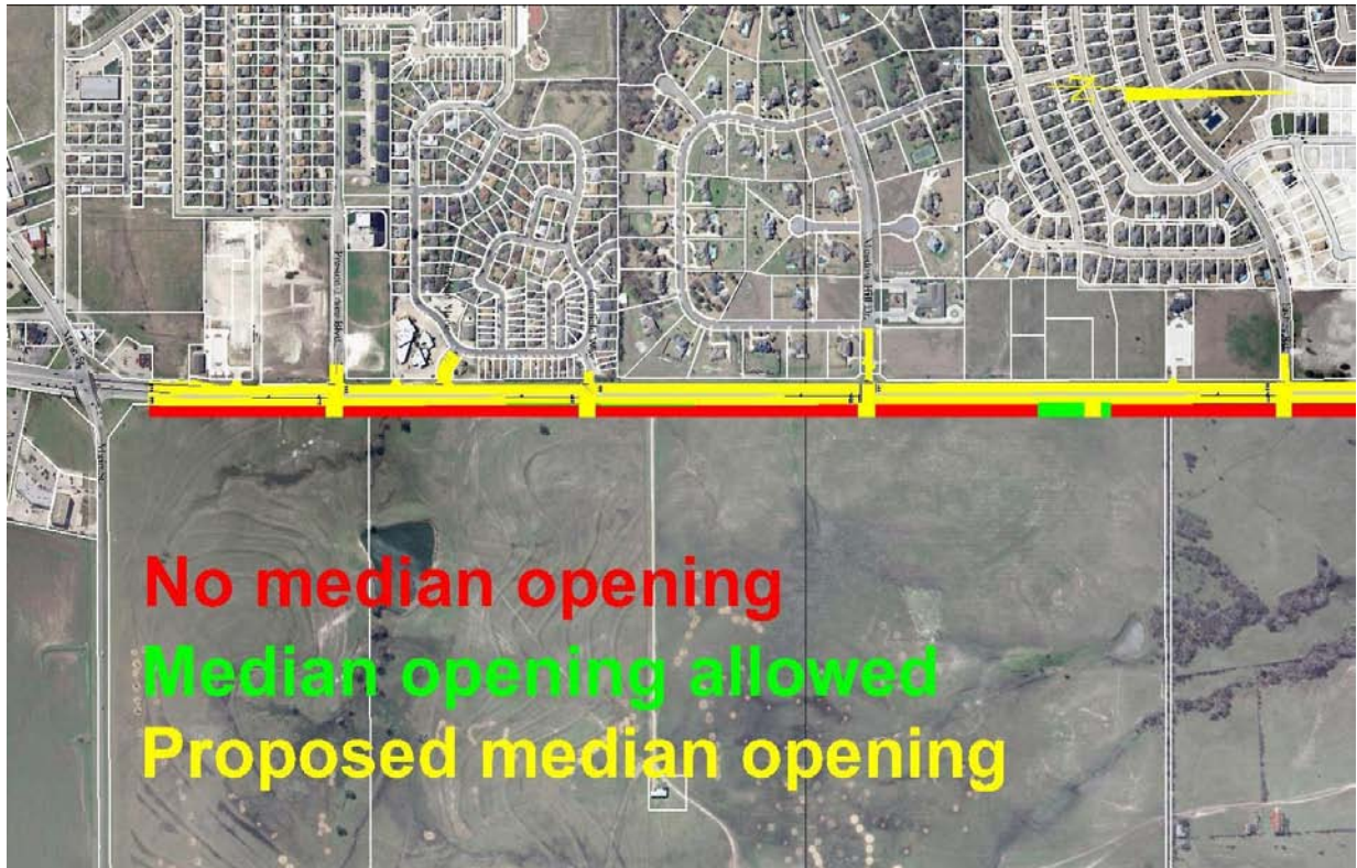
Figure 2 – Fine-Tuning of Median Openings
